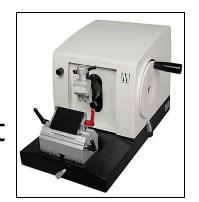
It holds the block of hard paraffin with the tissue in its center against a sharp metal knife that used to cut the block into thin sections (3-10 microns) as it moves up
