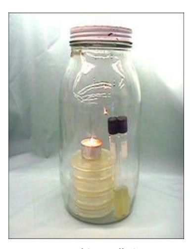
Anaerobic candle jar
