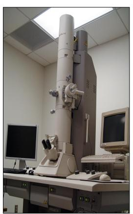
The lenses are electromagnetic coils instead of glass lenses
