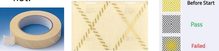
The color-changing indicator of tape is usually lead carbonate based, which decomposes to lead(II) oxide
