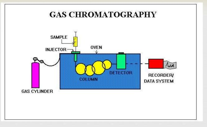
solution sample that contains organic compounds of interest is injected into the sample port where it will be vaporized. The vaporized samples that are injected are then carried by an inert gas (the mobile phase). The stationary phase is a microscopic layer of liquid inside a piece of glass or metal tubing called a column.
