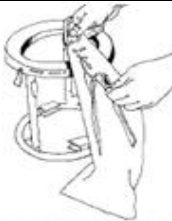
INDIVIDUAL SERVICE MEMBER FIELD TOILET
