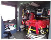
Figure 22.7 HEMS helicopter interior (a) Eurocopter EC135 T3 air ambulance. (b) Interior of EC135 showing attendants seat and patient stretcher.
