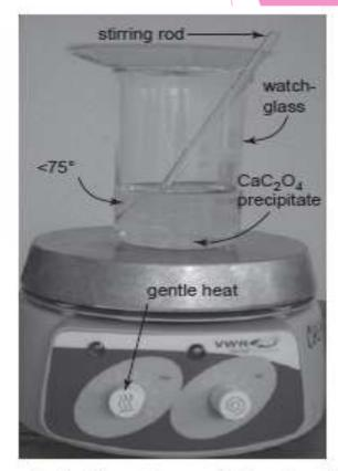
Figure 8.1 Warming and digesting the precipitate.
