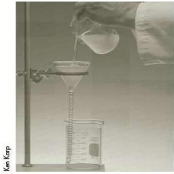
Figure 8.2 Gravity filtration is used to filter finely divided precipitates.
