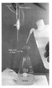
**Figure T.16j** Place a white background beneath the receiving flask and wash the wall of the receiving flask periodically during the titration.
