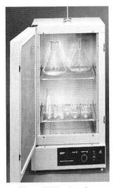
Figure T.15a A modern laboratory drying oven.
