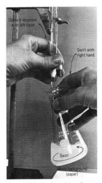
Figure T.16h Titration technique for right-handers.
