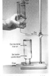
Figure T.8b Collection of water-soluble gases less dense than air.
