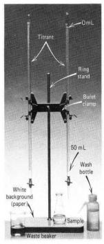
Figure T.16f Setup for a titration analysis.
