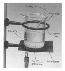
Figure 5.1 Warming and digesting the precipitate
