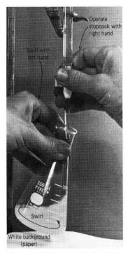
**Figure T.16i** Titration technique for left-handers.
