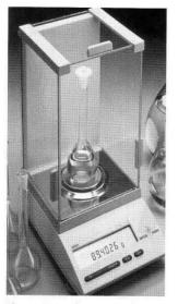
**Figure T.6c** Electronic analytical balance, sensitivity of  $\pm 0.0001$  g.
