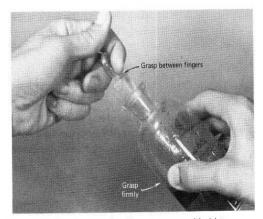
Figure T.10a Remove the glass stopper and hold it between the fingers of the hand that grasps the reagent bottle.
