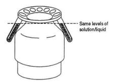
**Figure T.11i** Balance the centrifuge by placing tubes with equal volumes of liquid opposite each other inside the metal sleeves of the rotor.
