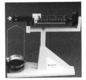
Figure T.6a Triple-beam balance, sensitivity of  $\pm 0.01$  g.
