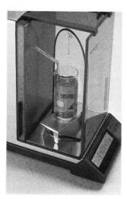
**Figure T.6d** Electronic analytical balance, sensitivity of ±0.00001 g.
