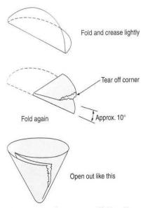
**Figure T.11c** The sequence of folding filter paper for a filter funnel in a gravity filtration procedure.
