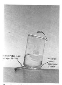
**Figure T.11a** Tilt the beaker to allow the precipitate to settle at the side. Use a stirring rod or a similar object to tilt the beaker.
