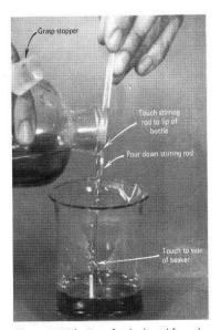
Figure T.10b Transfer the liquid from the reagent bottle with the aid of the stirring rod.
