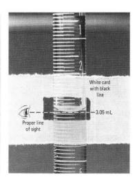
**Figure T.16b** Use a black line drawn on a white card to assist in pinpointing the location of the bottom of the meniscus.
