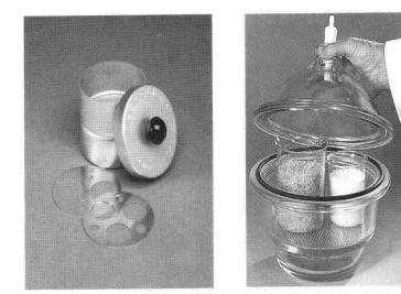
**Figure T.15b** A simple laboratory desicooler (left) or a glass desiccator (right) contains a desiccant (usually anhydrous CaCl<sub>2</sub>) to provide a dry atmosphere.
