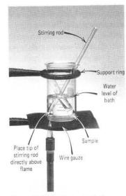
**Figure T.13d** A hot water bath may be used to maintain solution in test tubes at a constant, elevated temperature for an extended time period.
