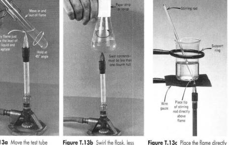
Figure T.13a Move the test tube circularly in and out of the cool flame, heating the liquid or solution from top to bottom.
