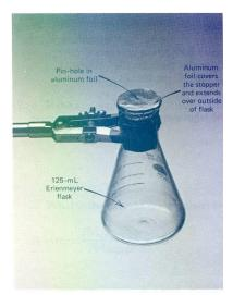
**Figure 3.1.** Preparation of a flask for the placement of the volatile liquid
