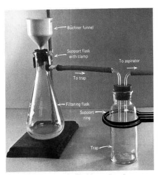
**Figure T.11f** The aspirator should be fully open during the vacuum filtering operation.
