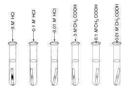
Figure 6.7 A setup for testing the effect of different acids and acid strengths on their reactivity with a meta
