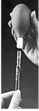
**Figure T.16c** Draw the liquid into the pipet with the aid of a rubber pipet bulb (*not* the mouth!).
