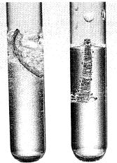
Hydrogen gas is produced at different rates from the reaction of zinc metal with hydrochloric acid (left) and phosphoric acid (right).
