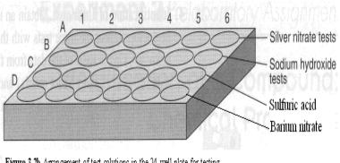
Figure 3.2b Arrangement of test solutions in the 24-well plate for testing salts
