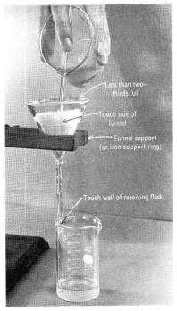
Figure T.11d The tip of the funnel should touch the wall of the receiving flask, and the bowl of the funnel should be one-half to twothirds full.
