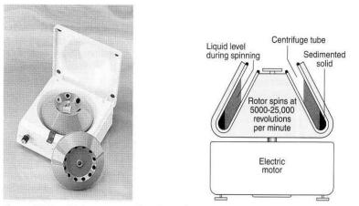
Figure T.11g A laboratory centrifuge forces the precipitate to the bottom of the centrifuge tube.
