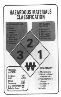
Figure T.3b Hazardous materials classification system.
