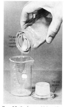
Figure T.9a Transferring a solid chemical from a glass ground reagent bottle. Place the glass stopper top side down.
