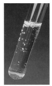
**Figure 3.1** A reaction mixture of NaHCO<sub>3</sub>(aq) and HCl(aq) produces CO<sub>2</sub> gas.
