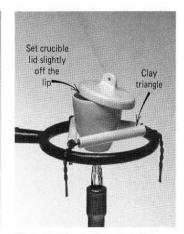
Figure T.15e Ignition of a solid sample in the presence of air for complete combustion.
