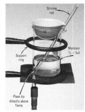
Figure T.14b Evaporation of a nonflammable liquid over a steam bath. A hot plate may be substituted for the flame.
