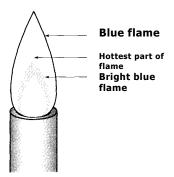
**Figure 1.3** Flame of a properly adjusted Bunsen burner.
