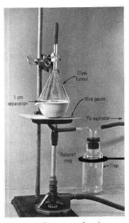
Figure T.12b Position a funnel, connected to a water aspirator, over the escaping gases.
