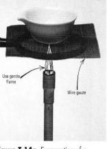
Figure 1.14a Evaporation of a nonflammable liquid over a low, direct flame. A hot plate may be substituted for the flame.
