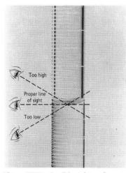
Figure **1.16a** Read the volume of a liquid with the eye horizontal to the bottom of the meniscus.
