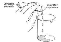
Figure T.11h Decant the supernatant from the compacted precipitate.
