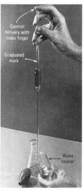
**Figure T.16d** Control the delivery of the liquid from the pipet with the forefinger (*not* the thumb!).
