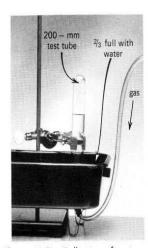
Figure T.8c Collection of waterinsoluble gas by the displacement of water.
