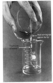
**Figure T.10c** The stirring rod should touch the lip of the transfer vessel and the inner wall of the receiving vessel.
