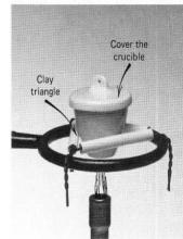
Figure T.15d Ignition of a solid sample in the absence of air.
