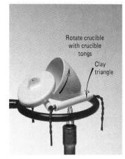
**Figure T.15c** Drying and/or firing a crucible and cover.
