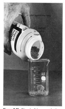
**Figure T.9b** Tilt and roll the reagent bottle back and forth until the desired amount of solid chemical has been dispensed.
