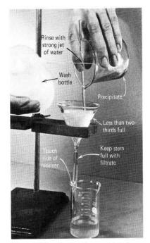
**Figure T.11e** Flushing the precipitate from a beaker with the aid of a "wash" bottle.
