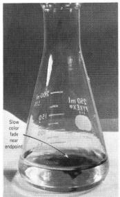
**Figure T.16k** A slow color fade of the indicator occurs near the endpoint in the titration.
