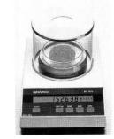
Figure T.6b Electronic top-loading balance, sensitivity of  $\pm 0.01$  g and/or  $\pm 0.001$  g.
