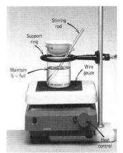
Figure T.14c Evaporation of a flammable liquid over a steam bath using a hot plate for the heat source.
