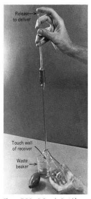
Figure T.16e Deliver the liquid from the pipet with the tip touching the wall of the receiving flask.
