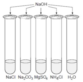
**Figure 2.3** Arrangement of test tubes for testing with the sodium hydroxide reagent.
