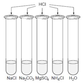
**Figure 2.4** Arrangement of test tubes for testing with the hydrochloric acid reagent.
