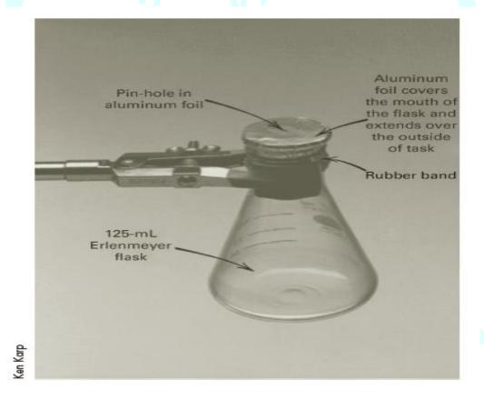
Preparation of an E/M flask for the placement of a volatile liquid
