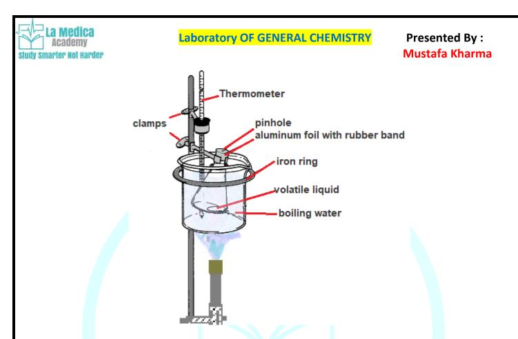
Apparatus for determining the molar mass of a volatile liquid.
