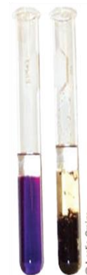
Hexane does not react with purple \text{KMnO}_4 (left); cyclohexene (right) reacts, producing a brown-black precipitate of \text{MnO}_2 .
