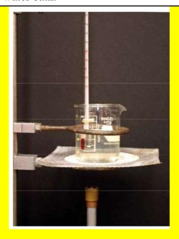
Figure. Boiling point apparatus
