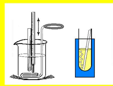
When a rapid and continuous stream of bubbles comes out of the small capillary tube and passes through the liquid, discontinue heating and allow the apparatus to cool.
