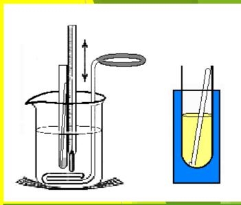
When the bubbles stop coming out of the capillary tube and just before the liquid enters it, read the temperature on the thermometer. This temperature is the boiling point of the liquid.
