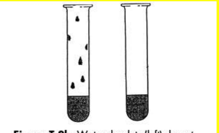
Figure T.2b Water droplets (left) do not adhere to the wall of clean glassware (right).
