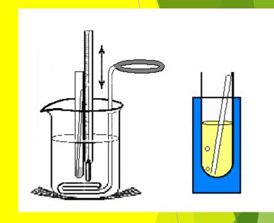
✓ While the system is being heated, bubbles will come out of the open end of the capillary tube.
