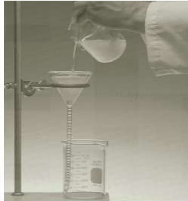
Figure 8.2 Gravity filtration is used to filter finely divided precipitates.
