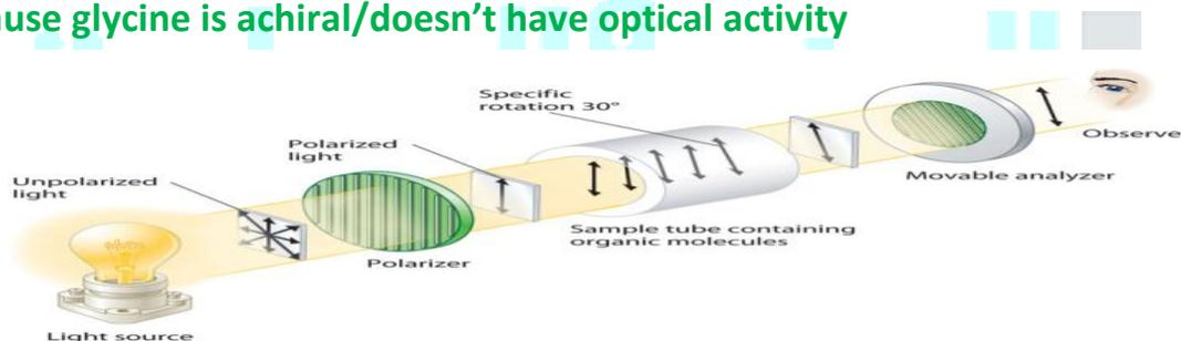
**Polarimeter is used to measure optical rotation**
