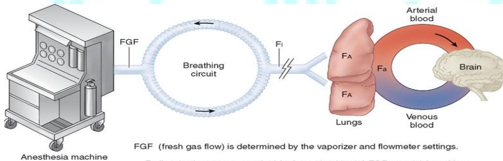
FGF (fresh gas flow) is determined by the vaporizer and flowmeter settings.
