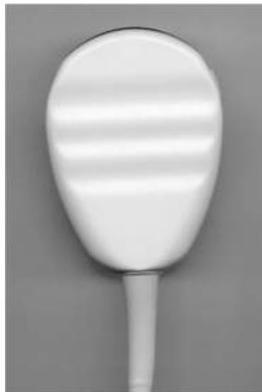
Figure 4.1 Ultrasound probe: abdominal.
