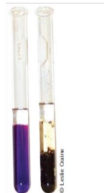
Hexane does not react with purple \text{KMnO}_4 (left); cyclohexene (right) reacts, producing a brown-black precipitate of \text{MnO}_2 .
