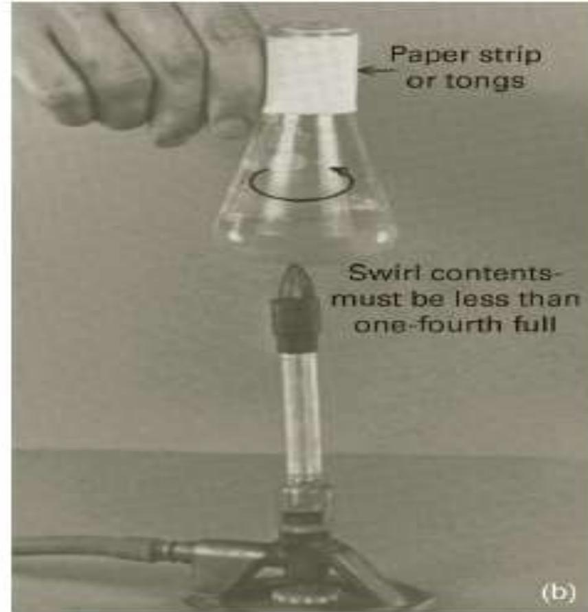
**Figure 17.2** Gently heat the sample to remove  $\text{CO}_2$  gas.
