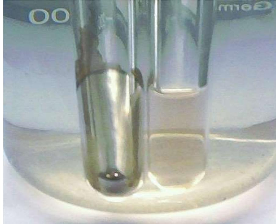
Figure 1: Tollens' test for aldehyde: left side positive (silver mirror), right side negative
