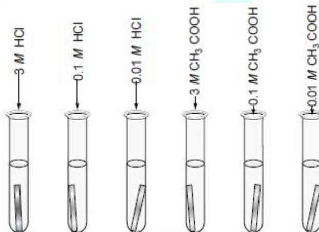
**Figure 6.7** A setup for testing the effect of different acids and acid strengths on their reactivity with a metal.
