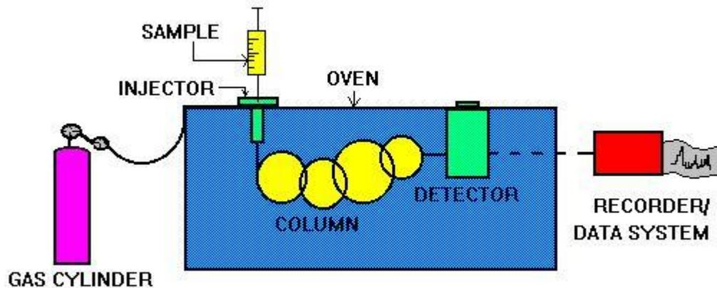
solution sample that contains organic compounds of interest is injected into the sample port where it will be vaporized. The vaporized samples that are injected are then carried by an inert gas (the **mobile** phase). The **stationary** phase is a microscopic layer of liquid inside a piece of glass or metal tubing called a column.
