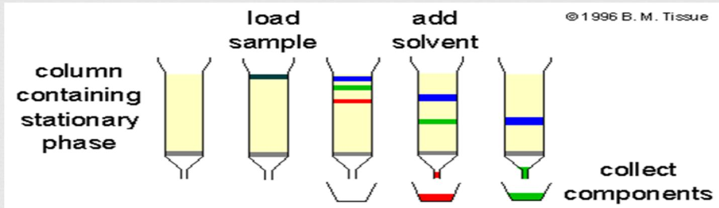
is a technique used to separate, identify, and quantify each component in a mixture. It relies on pumps to pass liquid solvent containing the sample mixture through a column filled with a solid adsorbent material. Each component in the sample interacts slightly differently with the adsorbent material, causing different flow rates for the different components and leading to the separation of the components as they flow out of the column.
