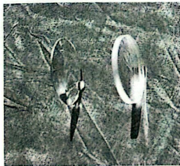
FIGURE 23-31 (a) Converging lenses and (b) diverging lenses, shown in cross section. Converging lenses are thicker at the center whereas diverging lenses are thicker at the edges. (c) Photo of a converging lens (on the left) and a diverging lens (right). (d) Converging lenses (above), and diverging lenses (below), lying flat, and raised off the paper to form images.
