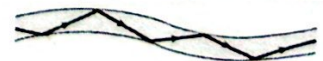
FIGURE 23-29 Light reflected totally at the interior surface of a glass or transparent plastic fiber.
