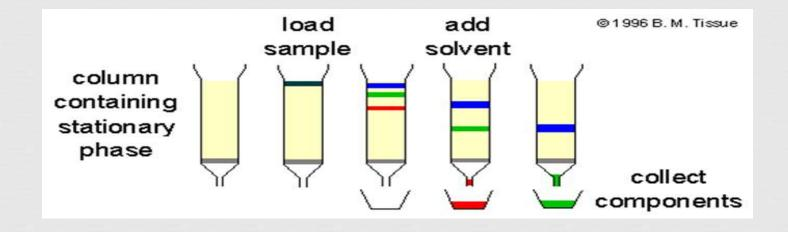
is a technique used to separate, identify, and quantify each component in a mixture. It relies on pumps to pass liquid solvent containing the sample mixture through a column filled with a solid adsorbent material. Each component in the sample interacts slightly differently with the adsorbent material, causing different flow rates for the different components and leading to the separation of the components as they flow out of the column.
